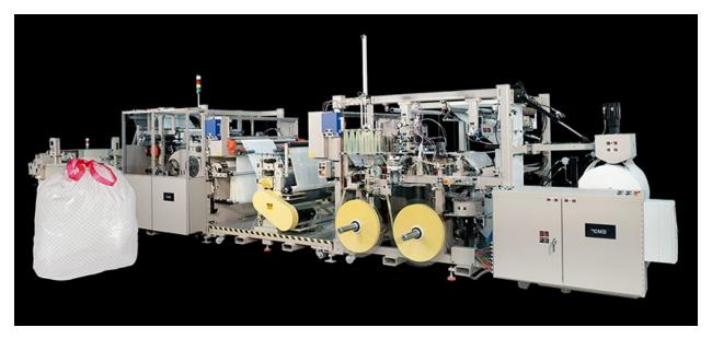
The systems allow for high-speed production of high-quality, premium drawtape trash bags on overlapped/interleaved rolls, where each bag is wound on top of the other, providing easy, one-at-a-time dispensing of the bag from the roll – a market offering that aligned very well with TPBI's commitment to value-added products as an important component of their product mix.
