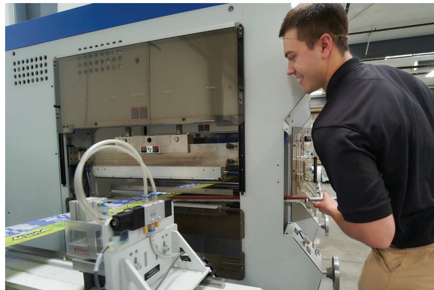
The CMD 760 Stand Up Pouch System design allows for die changes within minutes, significantly reducing downtime and waste.
