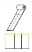
In overlap mode, the perforation connecting the bags is broken, and each bag is "overlapped" onto the next bag, so it is not necessary to tear one bag from the web when dispensing a bag from the roll.
